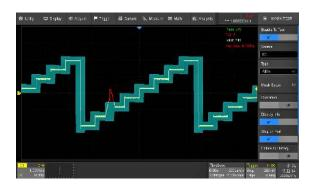
The T3DSO3000 utilizes a hardware based mask test function, that can perform 18,000 pass/fail tests per second. Users can define their own masks directly from a waveform or from the mask editor capability. The masks can then be used for Go/No Go testing with any failures stored as history waveforms or screen shots. The masks can also be stored on the T3DSO3000 for future use, making it suitable for long-term signal monitoring or automated production line testing.
