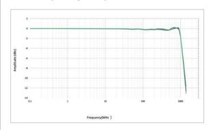
T3DSO31004 at 5 GSa/s shows exceptionally flat frequency response up to its maximum 1 GHz bandwidth.
