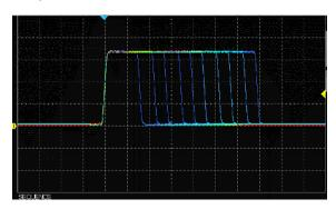
Segmented memory mode can store up to 100,000 waveforms into memory segments for capturing fast events in quick succession. Combine Sequence Mode with advanced triggers to isolate rare events. All the segments can be play back using the History function.
