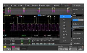
Simultaneously trigger and decode up to 2 common embedded and automotive serial buses, I<sup>2</sup>C, SPI, UART, LIN, CAN, CAN FD, FlexRay, I<sup>2</sup>S, MIL-STD-1553B, SENT and Manchester. Protocol information can be quickly and intuitively displayed, time aligned with the waveform and in table format.
