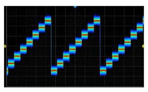
The Color temperature display clearly shows noise and jitter with infrequently occurring waveforms shown in blue through to the most frequently occurring waveforms shown in red.
