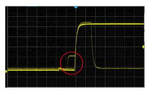
With a waveform capture rate of up to 500,000wfm/s (sequence mode) and 110,000 wfm/s (normal mode) the T3DSO3000 can easily capture glitches, infrequent anomalies and other low-probability events.
