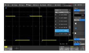
The always enabled History mode records up to 100,000 waveforms allowing users to scroll back through previous acquisitions to analyze past events and locate anomalies quickly. Serial decode, zoom and cursor measurements can be used.
