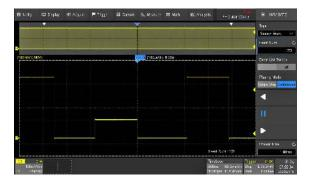
The T3DSO3000 can find events within an acquisition record or history acquisition based on user specified trigger conditions. Navigate browses through Events flagged by the Search, plays back history events or continuously moves the delay position on long records (very useful in zoom view).
