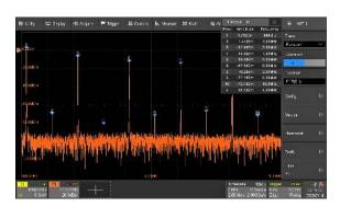
Two Math traces support Plus, Minus, Multiply, Divide, FFT, integration, differential, square root, and formula editor, providing a quick insight into the waveform characteristics.
