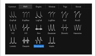
The optional 25 MHz function/arbitrary waveform generator comprises 6 standard waveforms and 45 arbitrary waveforms.
