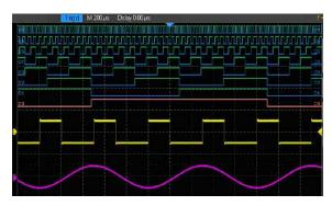
The MSO option adds 16 digital channels to the T3DSO3000 enabling users to trigger and acquire digital as well as analog waveforms in a mixed signal debug environment.
