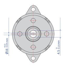
The FDT-70B-903 has a slotted groove which is excellent for usage with spiral springs
