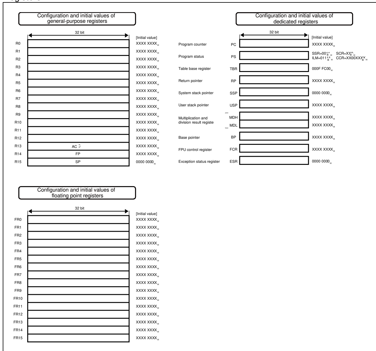
Figure 8-1 Initial Values of General-purpose Registers, Dedicated Registers, and Floating Point Registers
