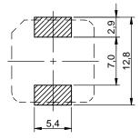
no sensitive traces underneath the component
