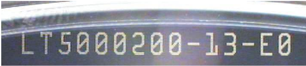
Figure 3-2. Wafer Identification Code 1
