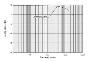
■ Differential Mode Transmission Characteristics (Typ.) **DLP11SA Series**
