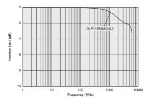
■ Differential Mode Transmission Characteristics (Typ.) **DLP11RB Series**
