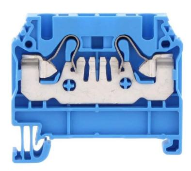
Feed-through terminal, Push-in connection, Mounting type: Mounting rail TS 35/7.5, Rated cross-section: 4 mm², Width: 6.1 mm, Colour: Blue
