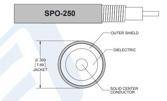
SPO-250 Coax Using Times Microwave Parts PE3C6346-100CM
