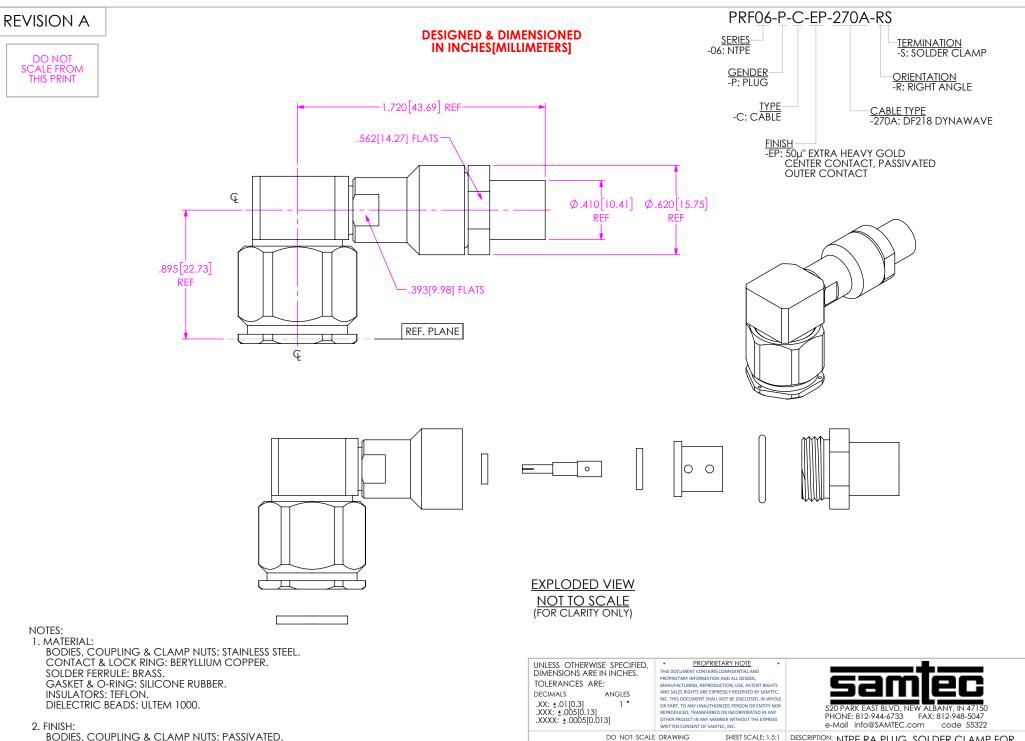
BODIES, COUPLING & CLAMP NUTS: PASSIVATED. CONTACT & SOLDER FERRULE: GOLD OVER NICKEL PLATE, 50 µIN MIN GOLD OVER 50 µIN MIN NICKEL.
