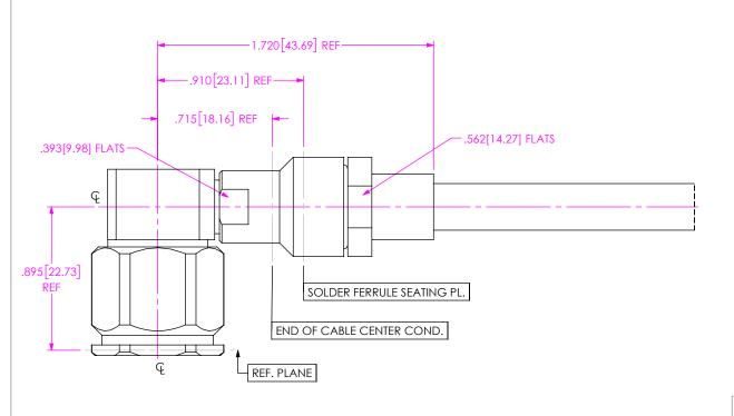
5. INSERT CABLE/CONTACT SUB-ASSEMBLY INTO CONNECTOR UNTIL SEATED AND TIGHTEN CLAMP NUT TO 35-45 IN-LBS.
