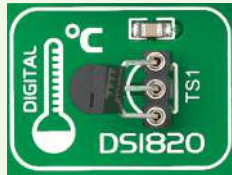
Figure 20-2: DS1820 correctly placed in socket
