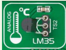
Figure 21-2: LM35 correctly placed in socket
