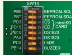
Figure 21-3: Enabled SW14.7 DIP switch
