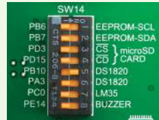
Figure 20-3: Enabled SW14.5 DIP switch
