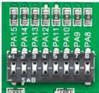
Figure 6-2: Tri-state DIP switch on PORTA/H
