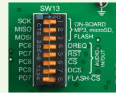
Figure 14-2: Enabling audio codec communication lines
