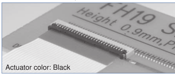
FH19S Series – FPC, FFC thickness: 0.3 \pm 0.03\text{mm}
