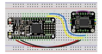
Board 3V to PCF8591 VIN (red wire) Board GND to PCF8591 GND (black wire) Board SCL to PCF8591 SCL (yellow wire) Board SDA to PCF8591 SDA (blue wire) PCF8591 A0 to PCF8591 Out
