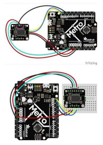
Connect PCF8591 VCC (red wire) to Arduino 5V if you are running a 5V board Arduino (Uno, etc.). If your board is 3V, connect to that instead. Connect PCF8591 GND (black wire) to Arduino GND Connect PCF8591 SCL (yellow wire) to Arduino SCL Connect PCF8591 SDA (blue wire) to Arduino SDA For our test program, we expect you'll wire up the ADC / DAC pins as well:
