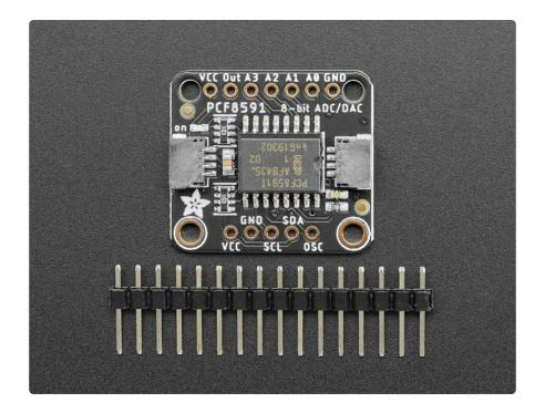
Along with four 8-bit ADC channels, the PCF8591 comes complete with an 8-bit Digita I to Analog Converter converter as well! Not only can you measure voltages, but now you can create them just as you want them. You can even use the DAC and ADC together to create an input to a circuit and measure the results with the ADC. The possibilities abound!
