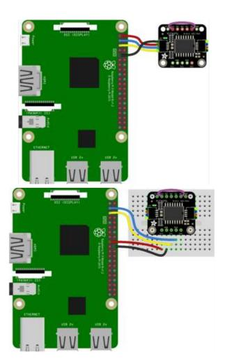
Board 3V to PCF8591 VIN (red wire) Board GND to PCF8591 GND (black wire) Board SCL to PCF8591 SCL (yellow wire) Board SDA to PCF8591 SDA (blue wire) PCF8591 A0 to PCF8591 Out
