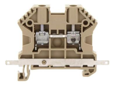
Feed-through terminal, Screw connection, Mounting type: Mounting rail TS 35/7.5, Rated cross-section: 4 mm<sup>2</sup>, Width: 6 mm, Colour: Orange
