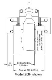
CAUTION: Downward tension on signal cable can cause wheel(s) to lift. Make sure cable is clamped to machine frame near encoder and allow slack.
