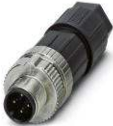
Sensor/actuator connector, plug, straight, 4-pos., M12 SPEEDCON, A-coded, spring-cage connection, metal knurl, cable diameter max. 8 mm
