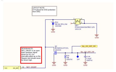
To conserve power, the onboard cellular module does not automatically startup when power is applied. The baseboard design must supply a means to assert a logic-low level on the ON\_OFF pin. To initiate the startup procedure, tie ON\_OFF to ground for at least 500 ms.
