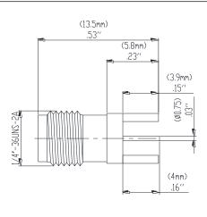
Model 72970 SMA STRAIGHT JACK PCB RECEPTACLE EDGE MOUNT
