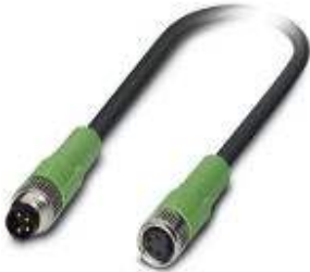
Sensor/Actuator cable, 4-position, PVC, Black RAL 9005, Plug straight M8, on Socket straight M8, Cable length: 1 m
