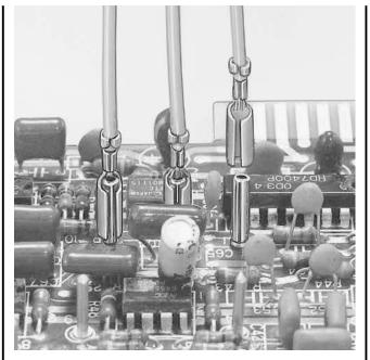
This connector is used with 2.36 mm diameter GT pins. The SPF connector has a large contact area, withstands stress caused by repeated insertions and removals, and provides excellent retaining force. It is best suited for circuit connections that require a large current.
