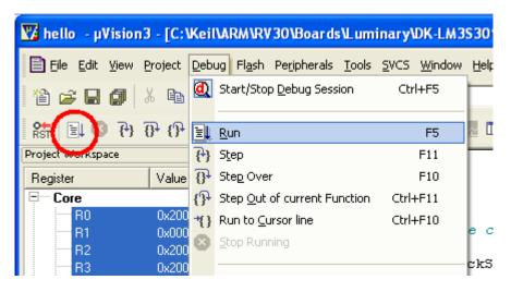
4. The application starts running, and you should see the text "Hello World!" output to the OLED display of the evaluation board.
