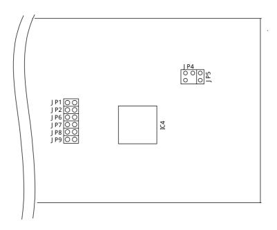
The following table shows the function of No 1 and No 2 of JP4, JP2, JP7. CU20049-UW2J is no reset inputs and M68 CPU bus parallel interface at default setting. Reset input signal is active when it is low.
