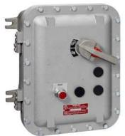
Non-reversing motor starter, Size 1, Three phase full voltage, Solid-state overload relay, OLRelay amp range 5.5-22a, 110 120/220 240VAC 60HZ coil, Combination type, 30Amp fusible disconnect 30 Amp /250V fuse clip, Encl. NEMA type 4X Fiberglass Water/dust tight noncorrosive, Standard width enclosure
