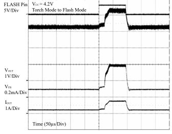
Figure 7 Torch Mode to Flash Mode
