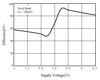
Figure 9 Supply Voltage vs. Efficiency (Torch Mode)
