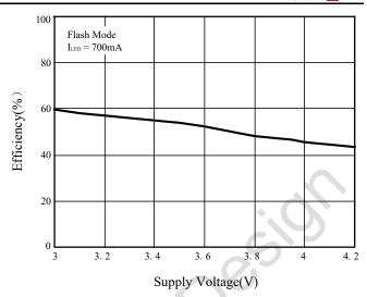
Figure 10 Supply Voltage vs. Efficiency (Flash Mode)
