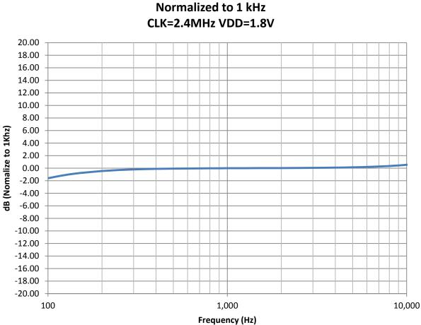
Typical Free Field Response Normalized to 1 kHz
