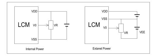
$V_{\text{DD-}}V_0\text{: LCD Driving voltage}$ VR: 10k~20k
