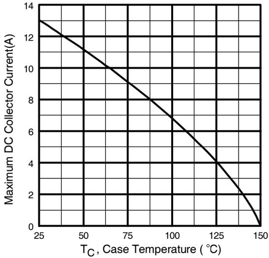
**Fig. 4 - Maximum Collector Current vs. Case Temperature**
