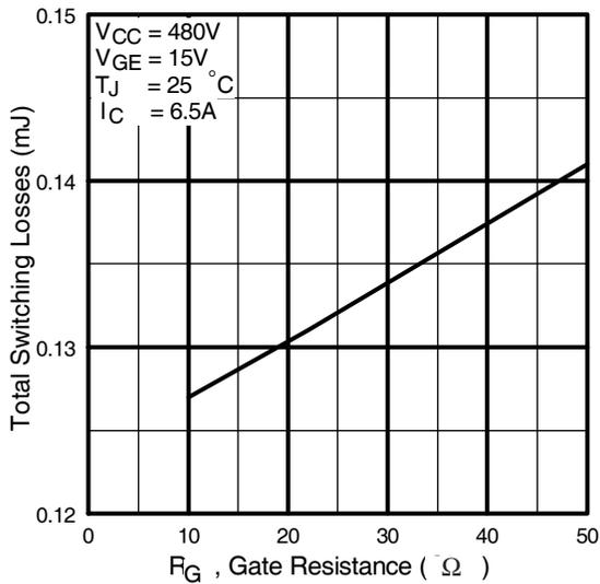
**Fig. 9** - Typical Switching Losses vs. Gate Resistance
