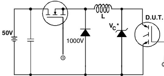
\* Driver same type as D.U.T.;  $V_c = 80\%$  of  $V_{ce(max)}$
