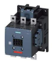
power contactor, AC-3e/AC-3 265 A, 132 kW / 400 V AC (50-60 Hz) / DC Uc: 200-277 V PLC input 24 V DC 3-pole, auxiliary contacts 2 NO + 2 NC permanently mounted drive: electronic main circuit: busbar control and auxiliary circuit: screw terminal
