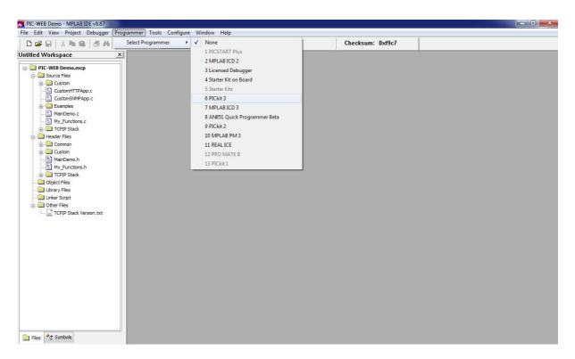
Wait while MPLAB is downloading operation system, and after Pic-Kit3 is connected – check in menu Programmer – Settings – Power – there is option – Power target circuit from PicKit3 – this option should be forbidden, you could not select it. Now it is safe to connect the programmer to your target board trough an ISCP cable. The PIC-WEB should be connected to the power supply.
