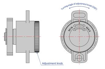
Turn the adjustment knob clockwise to increase damper torque and counterclockwise to decrease it.
