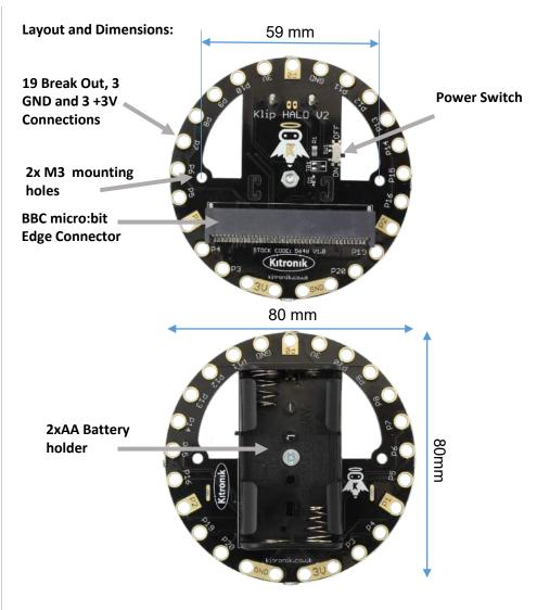
The Klip Halo board is 28.3mm thick (including BBC micro:bit connector and Battery holder)
