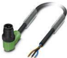
Sensor/Actuator cable, 3-position, PUR halogen-free, Black-gray RAL 7021, Plug angled M12, A-coded, on Free cable end, Cable length: 10 m, with plastic knurl
