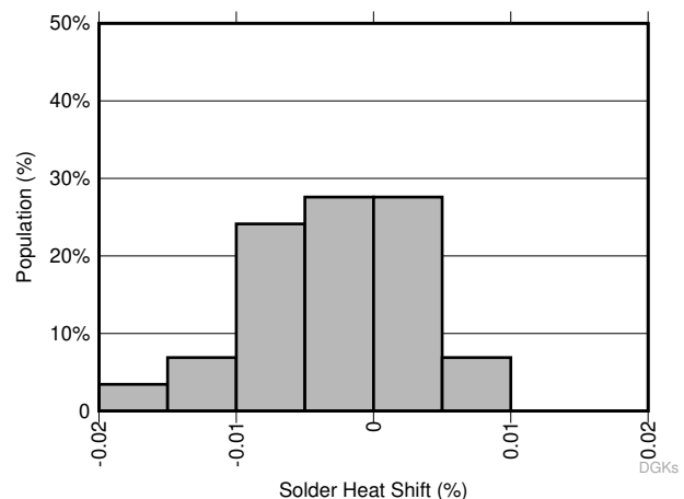
Figure 9-3. Solder Heat Shift Distribution, V_{REF} (%) - DGK Package
