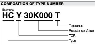
Resistance value, in ohm, is expressed by a series of six characters, five of which represent significant digits. The sixth R or K is a dual-purpose letter that designates both the value range (R for ohmic; K for kilo-ohm) and the location of decimal point.
