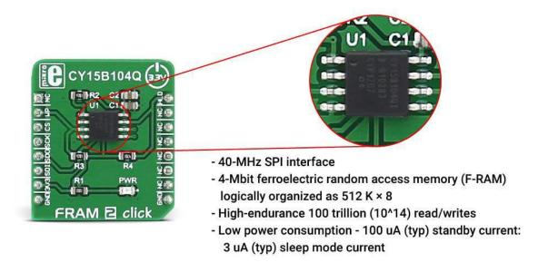
Unlike serial flash and EEPROM, the CY15B104Q performs write operations at bus speed. No write delays are incurred. Data is written to the memory array immediately after each byte is successfully transferred to the device.
