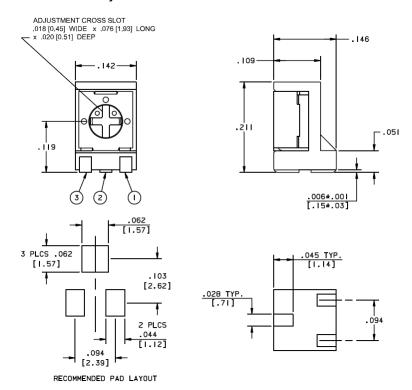
Dimensions are Inches [mm], Tolerances are ±.01 inch [±0.25 mm] unless otherwise stated.
