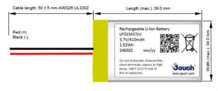
Thickness (max.): 3.5 mm (deliver status) 3.7 mm (after cycling)
