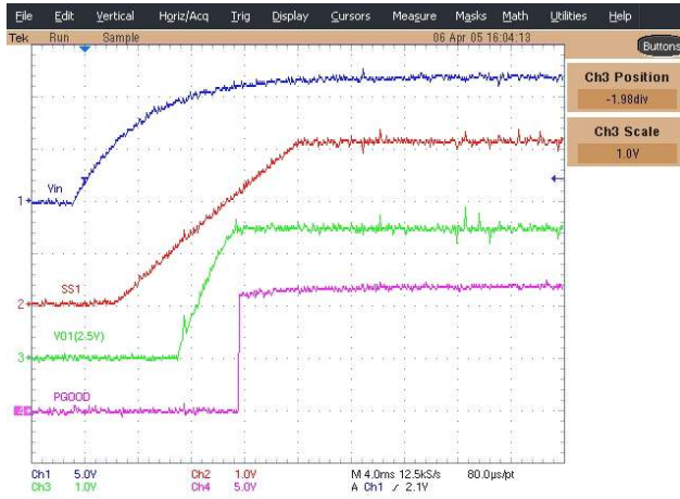
Figure 9 - 2.5V output Ch1: Vin, Ch2: SS1, Ch3: Vo1, Ch4: PGood
