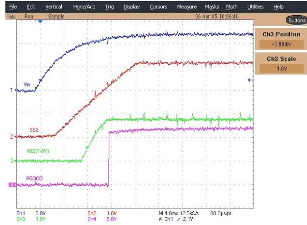
Figure 10 - 1.8V output Ch1: Vin, Ch2: SS2, Ch3: Vo2, Ch4: PGood
