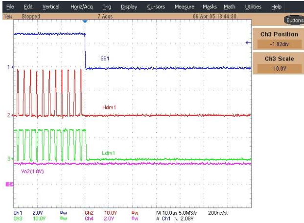
Figure 17 - SS1 pin shorted to Gnd Ch1: SS1, Ch2: Hdrv1, Ch3: Ldrv1, Ch4: Vo2
