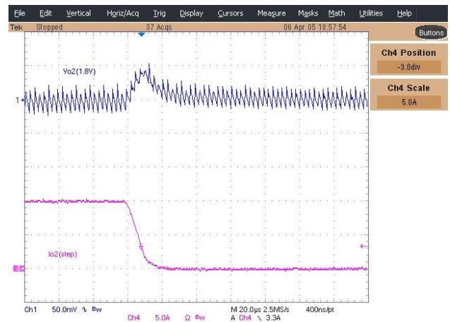
Figure 23 - Load Transient Respons for Vo2 ( I_o=10 to 0A) Ch1: Vo2, Ch4: Io2
