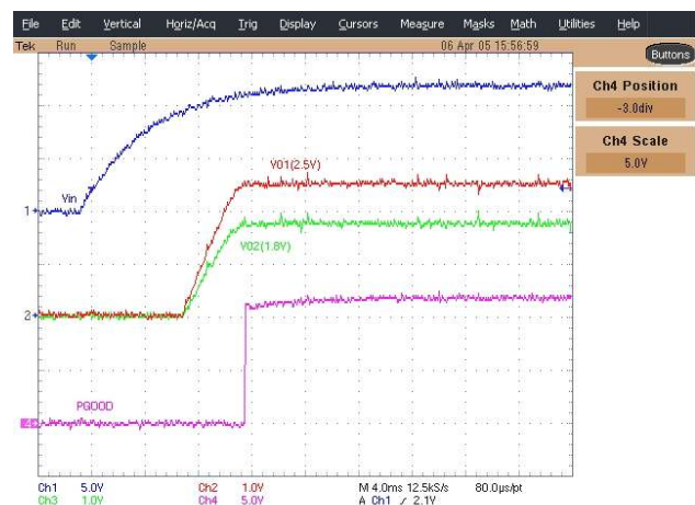
Figure 8 - Vo1, Vo2 and PGood Ch1: Vin, Ch2: Vo1, Ch3: Vo2, Ch4: PGood
