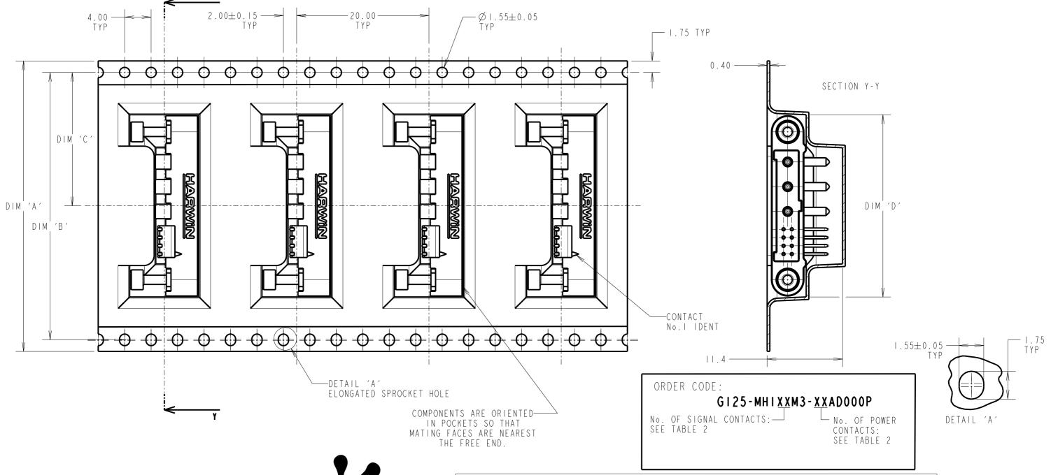
TABLE 2: AVAILABLE VARIANTS No. OF SIGNAL No. OF POWER DIM 'D' ASSEMBLY PART No. DIM 'A' DIM 'B' DIM 'C' CONTACTS CONTACTS G125-MH104M3-02AD000P 21.50 04 02 G125-MH108M3-03AD000P 08 03 44.00 40.40 20.20 27.60 G125-MH104M3-04AD000P 29.00 04 04 G125-MH124M3-02AD000P 34.00 24 02 G125-MH116M3-04AD000P 36.50 16 04 56.00 52.40 26.20 G125-MH108M3-06AD000P 39.00 08 06
