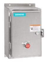
Non-reversing motor starter Size 1 Three phase full voltage Solid-state overload relay OLRelay amp range 3-12A 110VAC 50HZ / 120VAC 60HZ coil Combination type Water/dust tight non-corrosive
