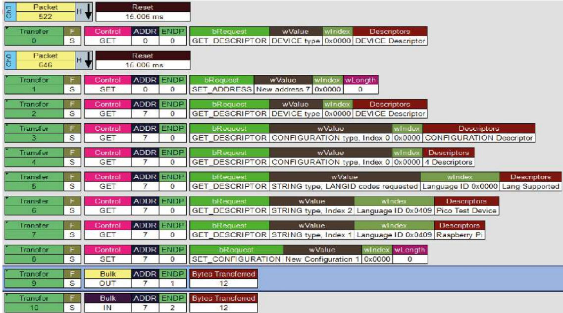
Figure 54. USB analyser trace of the dev_lowlevel USB device example. The control transfers are the device enumeration. The first bulk OUT (out from the host) transfer, highlighted in blue, is the host sending "Hello World" to the device. The second bulk transfer IN (in to the host), is the device returning "Hello World" to the host.
