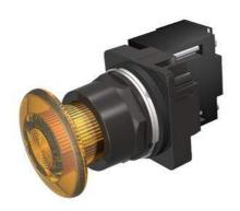
30mm BlackMax, Epoxy Coated Corrosion Resistant Complete Metal Unit Illuminated Push-Pull Operator Full Voltage, 6V AC/DC Incandescent Lamp Mushroom Head Cap Small 1 3/4" (44.5 mm) Plastic, Amber 3 Position Pull-Momentary/Push-Maintained UL Listed, CSA Certified NEMA 1,3,3R,4,4X,12,13 & Automotive Standards
