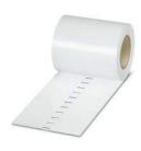
Marker for terminal blocks, can be ordered: by line, white, labeled according to customer specifications, mounting type: snap into universal marker groove, snap into flat marker groove, for terminal block width: 10.2 mm, lettering field size: 6.  $35 \times 10.15 \text{ mm}$
