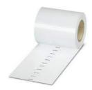
Marker for terminal blocks, Roll, white, unlabeled, can be labeled with: THERMOMARK ROLL 2.0, THERMOMARK ROLL, THERMOMARK ROLL X1, THERMOMARK ROLL MASTER 300/600, THERMOMARK X1.2, THERMOMARK S1.1, perforated, mounting type: snapped, snap into flat marker groove, for terminal block width: 10.2 mm, lettering field size: 6.35 x 10.15 mm, Number of individual labels: 10000
