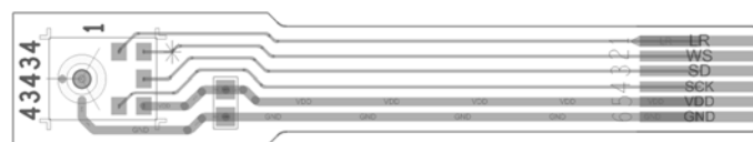
Figure 2. EV_ICS-43434-FX Evaluation Board Layout (Top View)
