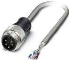
Bus system cable, DeviceNet, 5-position, PUR halogen-free, Gray RAL 7001, Plug straight 7/8"-16UNF, on Free cable end, Cable length: 2 m
