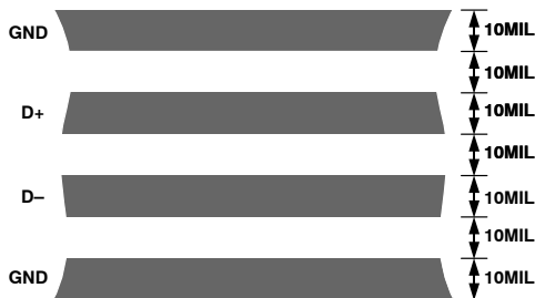
Figure 34. Arrangement of Signal Tracks
