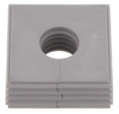
Seal, Mounting type: Plug in, Length x width: 42.8 mm, Max. cable diameter: 17 mm, IP 66, Colour: Grey
