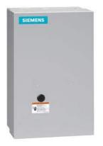
Electrically held lighting contactor, Contactor amp rating 30A, 0 N.C. / 6 N.O. Poles, 347VAC 60HZ coil, Non-combination type, (no disconnect device), Enclosure NEMA type 1, Indoor general purpose use
