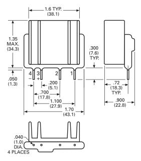
PIN ASSIGNMENTS: PIN 1: AC LOAD PIN 2: AC LOAD PIN 3: + DC INPUT PIN 4: - DC INPUT
