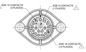
STANDARD DIA. WIRE SEAL SEALED PANEL MOUNT
