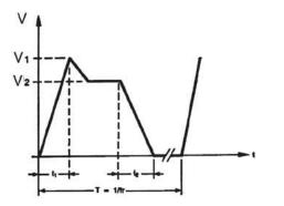
Choice of voltage:  $V_1 \le V_{peak}$  $V_2 \le V_n dc$ Maximum overvoltage  $\le V_s (10 \text{ s/day})$
